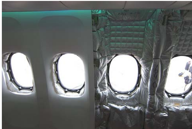
Insulation around the cabin windows of the Boeing 747-81 by Olivier Cleynen [CC-BY-SA-3.0], via Wikimedia Commons
