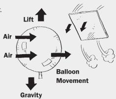
fanning at a balloon makes it hard to control the balloon's movement. Fanning results in chaotic air currents. They will move a balloon, but in an unpredictable way.
