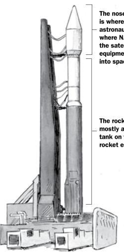
The nosecone is where the astronauts sit or where NASA stows the satellites or equipment it sends into space.
