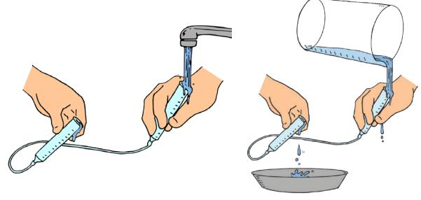
9. Instruct students to hold their systems level over a catch basin and push a plunger into one of the syringes. Excess water will flow out of the other syringe. Have them put the plunger back into the other syringe and press it down gently. (Remind students not to apply so much pressure that the other plunger pops out.) If the system was prepared properly, this motion will cause the plunger in the other syringe to retract.
