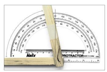
In this picture, the protractor is measuring an angle of 76 degrees. You read the smaller number because the angle is smaller than a right angle (90 degrees).
