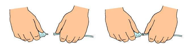
3. Once the systems are assembled, instruct students to push the retracted plunger completely into the syringe. This motion will push air through the tube and cause the plunger in the other syringe to retract.
