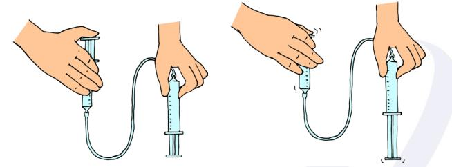
4. Tell students they've just created a system that uses air pressure to transfer motion. It is called a pneumatic system.
